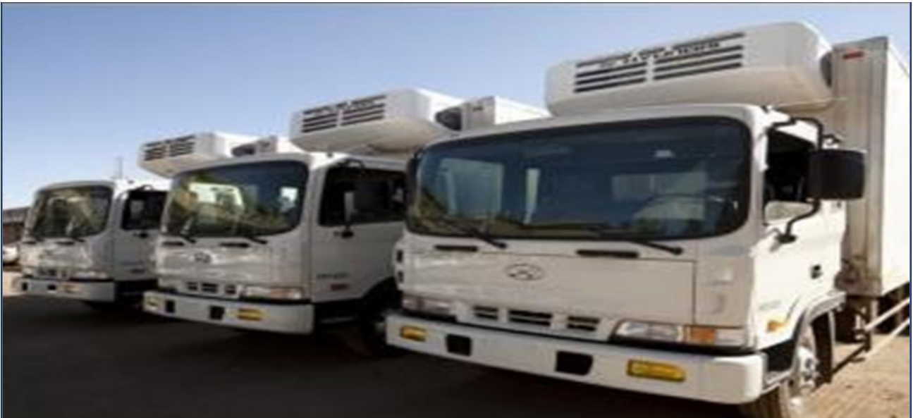
Figure 6-3 Refrigerated truck for vaccines
