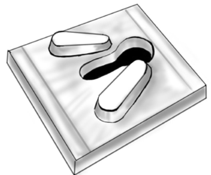
SanPlat concrete slab
