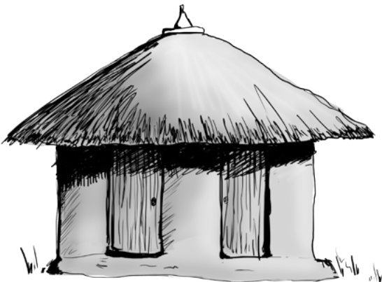
Figure 39: Mud plastered wooden wall/thatched roof
